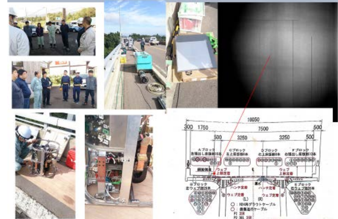
Third Bridge Inspection by 950 keV X-ray Source on Oct.6,7, 2016
